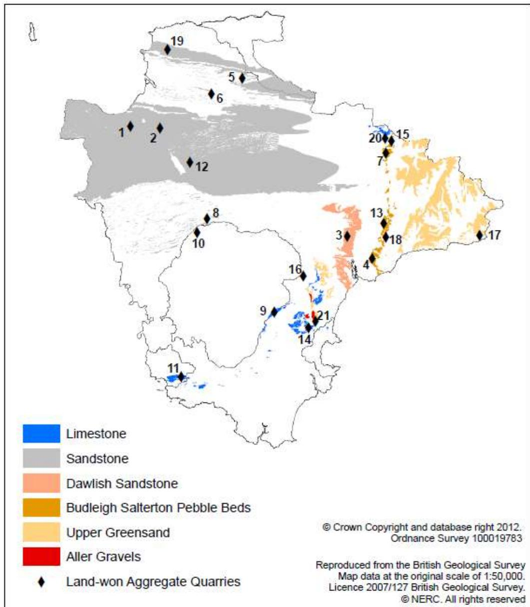
Figure 2.1: Location of currently-quarried geological formations and land-won aggregate quarries operational in 2011 (key to quarries in Appendix B)
